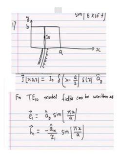
For only, z directed current we can write, surface current on the probe surface as **J**.
