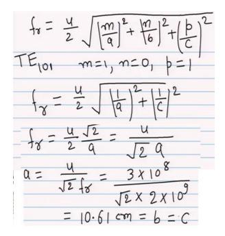
So, this will come 10.61 centimeter, so this is a that means equal to b equal to c so, this is the dimensions of the rectangular this cubical waveguide, cavity, cubical cavity.
