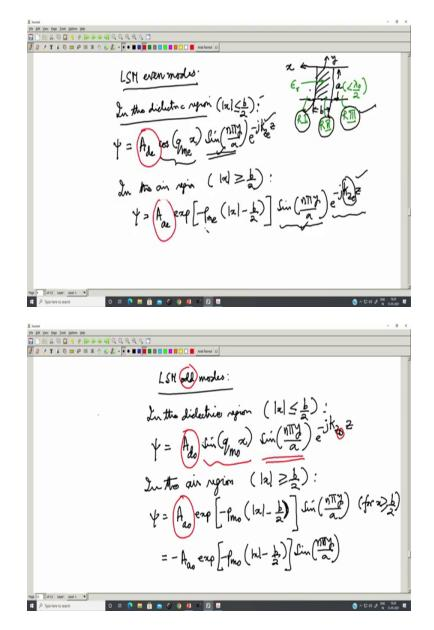
So, we have the two forms of the potential function for mod x, we have the two forms of the potential function for x greater than or equal to b/2 and x less than or equal to minus b/2.
