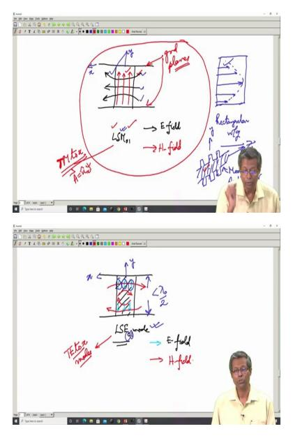
So, if I arrange the modes of the NRD in ascending order, the lowest one will be the  $LSE_{00}$  mode. So, this is frequency hertz, which has a 0 cut off frequency. So, it would propagate a dc followed by the  $LSE_{01}$  mode, which is the next higher order mode and then followed by the  $LSM_{01}$  mode, which is the next higher order modes. And then will come the other higher order NRD modes.
