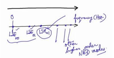
So, you see if we are preferentially using the LSM<sub>01</sub> mode, because of its low loss, we have to very well appreciate that there are two modes, LSE<sub>00</sub>, and LSE<sub>01</sub>, which have a lower cut off than the LSM<sub>01</sub>. And therefore these two modes will have a tendency to get generated at any kind of discontinuity surface imperfections of the NRD, curved sections and the like.
