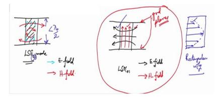
So, this is the electric field and magnetic field profile of the LSE<sub>01</sub> mode.
