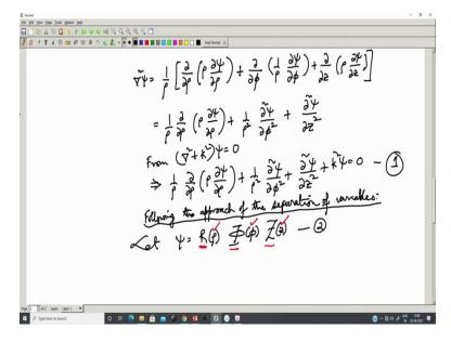
So, now, what we do is that substituting these values we get  $\nabla^2 \psi$  equal to  $\frac{1}{\rho} \left[ \frac{\partial}{\partial \rho} \left( \rho \frac{\partial \psi}{\partial \rho} \right) + \frac{\partial}{\partial \phi} \left( \frac{1}{\rho} \frac{\partial \psi}{\partial \phi} \right) + \frac{\partial}{\partial z} \left( \rho \frac{\partial \psi}{\partial z} \right) \right]$ . That is pretty much simple to understand.
