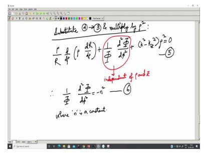
Now, we substitute 4 into 3 and multiply by rho squared. If we do that, we will obtain this equation  $\frac{\rho}{R} \frac{d}{d\rho} \left( \rho \frac{dR}{d\rho} \right) + \frac{1}{\Phi} \frac{d^2 \Phi}{d\phi^2} + \left( k^2 - k_z^2 \right) \rho^2 = 0$ . We call this equation 5. Now, we note that
