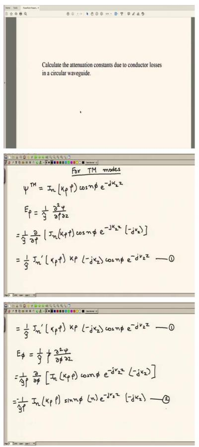
In the next question, we need to calculate the attenuation constants due to conductor losses in a circular waveguide. So, for finding out the attenuation constant, we will consider both the modes that is for TM modes and TE modes. So, to start with TM modes, we can write, Psi of TM as  $j_n(k_\rho\rho)\cos(n\phi)e^{-jk_z z}$ . Therefore, from the fields that we had previously found out that
