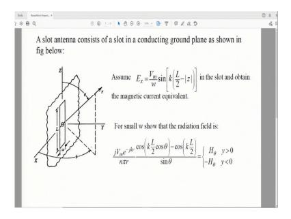
So therefore, we can then write **Ms** as  $\frac{2v_m}{w} \sin\left[k\left(\frac{L}{2}-|z|\right)\right]$ . So, this was the magnetic current equivalent. The first part is now obtained. Now what the second part says? It says that if we assume like w is very small then what will be the radiated fields?
