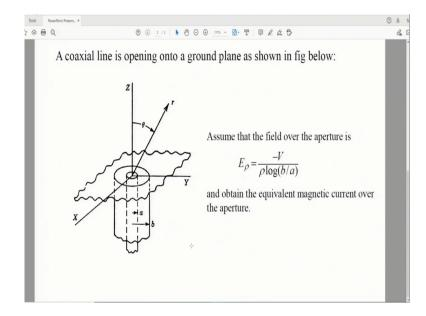
Now let us move to the next question. The next question says that there is one coaxial line up and it is opening onto a ground plane. So, here we have a coaxial line which is opening onto a ground plane. And again, it has been told that we need to assume that the field over the
