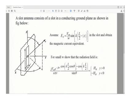
So, the first problem states that there is one slot antenna and it consists of a slot in a conducting ground plane as shown in the figure. So, there is a slot present. The length of the slot is given by L and the width is w and the length of the slot is along the z direction whereas the width of the slot that is w is along x- direction. It is assumed that Ex equals
