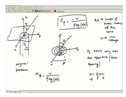
So, let us start solving this. So, it was given like we have a coaxial cable. This is the inner radius 'a' and this is the outer radius 'b'. This is z y x and we have a ground plane over here. This angle is theta. Now in the question it is asked, so basically this was our original problem given in the question. It was asked, it was told that the field over the aperture was given by, it
