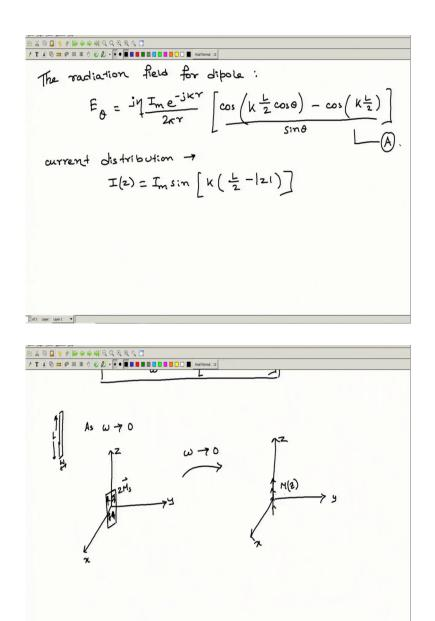
So, now we know that the radiation field for dipole, we can write, ok. For the current distribution of the radiation field can be written like  $E_{\theta} = \frac{j\eta I_m e^{-jkr}}{2\pi r} \left[ \frac{\cos\left(k\frac{L}{2}\cos\theta\right) - \cos\left(k\frac{L}{2}\right)}{\sin\theta} \right].$ So, this was the radiation field for dipole.
