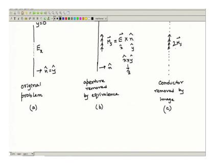
Now, then we can see like suppose, this was Ex, so this is the slot, this is Ex, so we can write this. So, this was our original problem. We have a slot on the conducting ground plane. So, this is our original problem, fine. So, here is the  $\frac{1}{h}$  is  $\frac{1}{y}$ , normal. Now this original problem, what we will do? By using the equivalence principle, we will replace the aperture by a patch of magnetic current.
