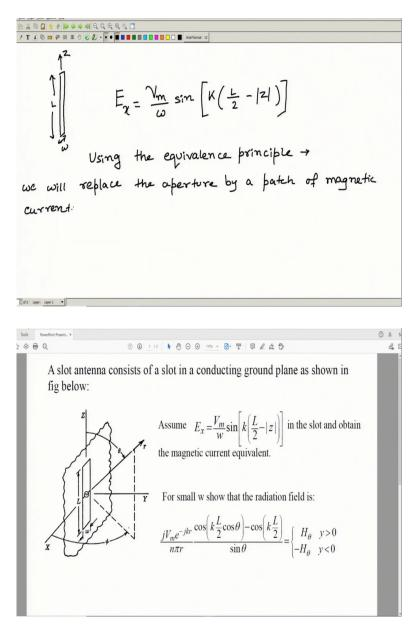
So, we are given a slot antenna. So, we will start with. So, basically, it is a dipole slot antenna when fed by a voltage that is impressed across the center of the slot. The slot and the ground plane, it can be viewed as a transmission line and the field in the slot will be essentially a harmonic function of  $k_z$ . So, basically, we were given a slot of length L and with w and this is z.
