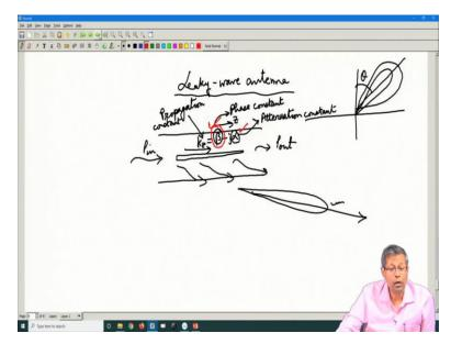
Let us suppose I will give you an example a Leaky-wave antenna; a Leaky-wave antenna. An example of a Leaky-wave antenna might be just a waveguide; so this is a waveguide, and on the narrow wall, I have cut a slot. This slot is not of uniform dimension; so the basic physics is as the waveguide is excited from the left hand side. So, this is the input port and this is the output port; energy radiates from this slot. So, we get we can get a pattern like this for instance.
