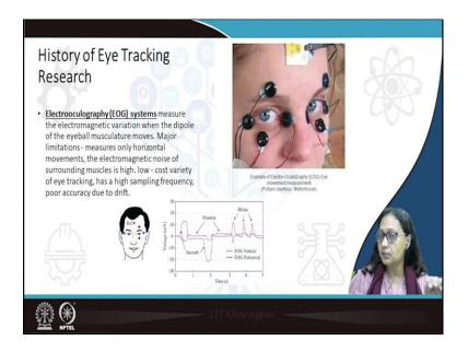
The next method that has been used is the electrooculography or electrooculogram as you often see. These the EOG systems they measure the electromagnetic variation when the dipole of the eyeball musculature moves.
