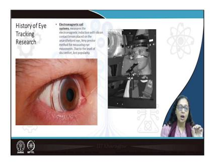
And the lenses systems have a very high precision, but are extremely uncomfortable. What they use is they introduce contact lenses for recording very detailed eye movements and one of these being the electromagnetic coil systems. Now this these electromagnetic coils they are actually silicon contact lenses placed in the anaesthetized eye.
