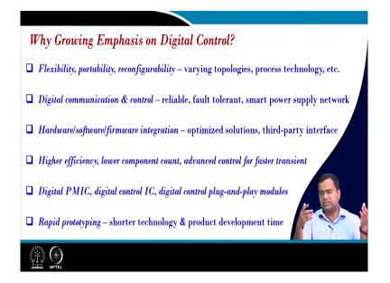
Now, where is where there is a growing trend for digital control? One of the reasons is that by using digital control we can make the design flexible; that means, as I said in the previous example the one IC can be used for various topologies; which means, we can program this IC through software and we can change the parameter we can configure it so that it can be used for other architecture or even it can be used for various power levels.
