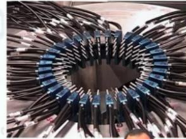
A fiber-optic array for detection of breast cancer by way of Diffuse Optical Tomography.
