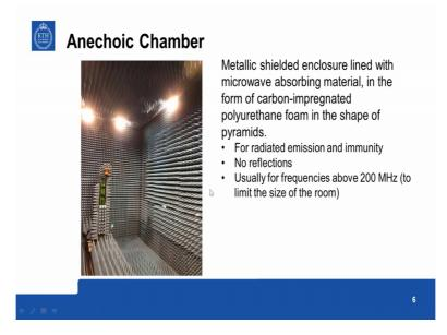
Anechoic Chamber, this is a metallic shielded enclosure lined with microwave absorbing material in the form of carbon-impregnated polyurethane form and these form are shaped like pyramid, so basically you have a shielded enclosure on the outside and the shield will prevent other electromagnetic fields from entering into the test area, so you are looking out all the external fields. Then the cones...the microwave absorbing materials will make sure that there are no reflections.
