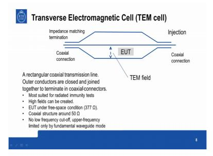
Another test equipment is TEM cell Transverse Electromagnetic Cell so here the principle is that you create a transverse electromagnetic field in a coaxial structure. We have seen what is meant by a TEM field while talking about uniform plane waves, transmission line et cetera, so this is actually a transmission line, a coaxial transmission line so this is formed by a rectangular metal chamber.
