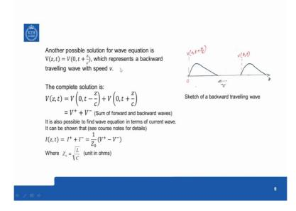
Another possible solution for wave equation is backward travelling wave so you can say that the wave that is present at z would be travelling backwards. So if it is a backward travelling wave it is this kind of reflection in transmission lines that we will see later, so it is T + (Z / V), so the total solution will be the sum of the forward travelling wave and the backward travelling wave. So we denote that by the symbols + and - in the superscript.
