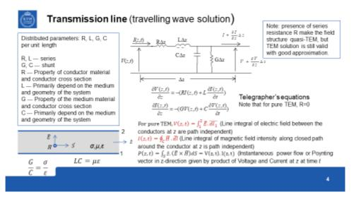
Now, first let us concentrate on this part trying to find the correspondence between the electric and magnetic fields with voltages and currents. So this is a transmission line structure; two parallel conductors so this is the length, the TEM wave is propagating along this Z direction, so E and H fields are perpendicular to the direction of propagation so let us assume the E vector to be like this and H vector is coming out of the paper let us say then this
