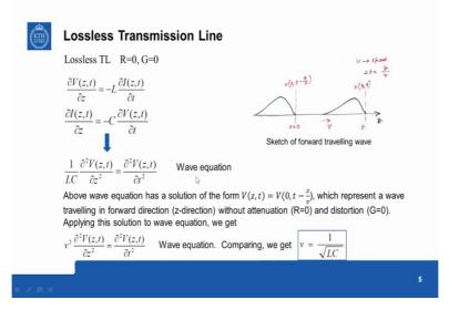
Now consider a lossless transmission line, it does not have any loss that is no attenuation that is R = 0 that is the amplitude are same, all around the transmission lines and load distortion G is equal to 0, no dissipation of the current along the way of the transmission line. So under this condition the previous equations simplify into these two equations, rate of change of
