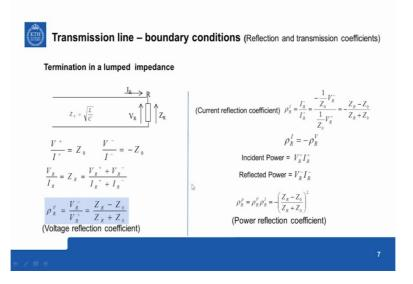
Now let us look at transmission lines boundary condition that is when transmission line is abruptly terminated either by a lumped impedance or it can be another transmission line that we will see in the next page. Suppose, it is terminated in a lumped impedance, and this reflection point here, so we call it as R so we call  $I_R$ ,  $V_R$  and  $Z_R$ ,  $Z_R$  is the impedance so  $V_R$  is the net voltage over here, so this is the sum of forward and backward reflected waves over
