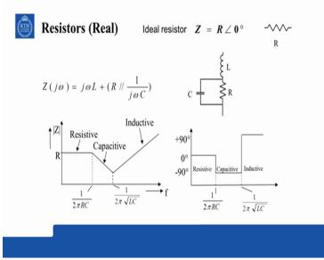
So then bode plot will be something like this. From resistance to capacitive it will go into. So depending upon the application area, depending upon the low value or high value of the resistor one of these two parasitic, one of these two bode plot will be more appropriate to be applied so two different models are possible for resistor.
