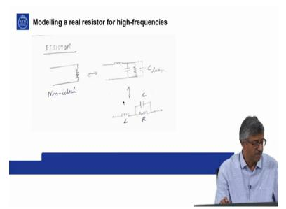
Now modeling a real resistor for high-frequencies, again we do the same exercise of including the parasitic elements of the component leads, inductor and capacitor. Or there can be a leakage capacitance across the register also which we can combine with this parasitic element. So you get circuit in which we have inductor, then we have a capacitor and resistor connected in parallel. So this will be the minimum model for a real resistor under high frequency.
