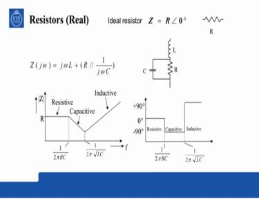
Consider a real resistor R, it has got due to the leads and due to the construction of the resistor some parasitic inductance L and some parasitic capacitance C. Now as the frequency is
