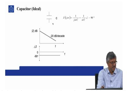
So we take the ideal capacitor. What is an ideal capacitor? Well, it has a symbol like this. So this is the ideal capacitor and it has a impedance which is a function of frequency. We know that it is 1 by J omega C or in polar form we write 1 by omega C and minus- 90. It means that the impedance is voltage divided by current. So voltage and current are 90 degrees face shifted and
