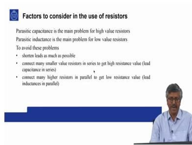
Factors to consider in the use of resistors: One is parasitic capacitance is main problem for high value resistors. Parasitic inductance is the main problem for low value resistors. To avoid these problems, shorten the leads as much as possible. When you reduce the parasitic elements both
