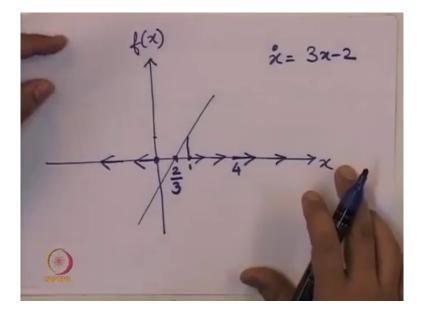
So, this particular point let me draw a slightly bigger figure, were considering the differential equation x dot is equal to 3 x minus 2 and we are going to plot f verses x even though x itself was a function of time and we will also later plot x as a function of time, but for now we are interested in drawing the vector field.
