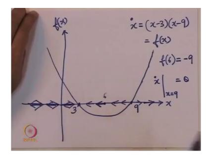
So, consider the differential equation x dot is equal to x minus 3 times x minus 9; which we want to call as f of x. So, this is equal to 3, this is equal to 9 and the graph of this function looks roughly like this. This function has roots at x equal to 3 and 9 and hence it is passing through 0 precisely at x equal to 3 and 9 and if we take a point 3, then we see that the vector at the point 3 has length 0 and hence we plotted neither to the right nor to the left.
