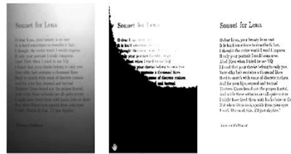
(a) Image with illumination gradient. (b) Global thresholding. (c) Local thresholding with correction for background/foreground only windows.
