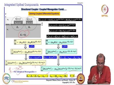
Now what do we do just once again I try to remind you if they are identical waveguide that means beta a = beta b = beta 0 kappa ab will be equal to this one kappa b star this one and delta beta 0 kappa a kappa bb delta beta 0 and delta will be equal to 0 that means I can directly put this one equal to 1 because the exponential 0 is 1 here also it will be 1. So, our solution will be very simple straightforward I can write dA by dZ = -j kappa ab B titled z.
