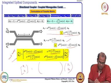
Now if I just try to make a matrix upon this is because A 0 B 0 is the input A 1 B 1 is output A 0 B 0 is the output I want A 1 B 1 that is this thing and some matrix form I will write so that I can get A 0 B 0 that is what do you need for circuit simulation. So, from this equation we can just simply write this is the A 1 component and this is coming from B 0. So, A 1 will be this one multiplied by A 0 plus this one multiplied by the one.
