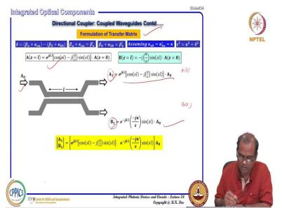
Now let us go for it we are now done that how to solve and how to design the waveguide obviously if you see that if you want a 3 dp power splitter kappa l should pi by 4 if it is pi by 4 that means sin kappa l = 1 by root 2 and sin square will be half. So, it will be 50% here and 50% here so you can design kappa l = pi by 4 or 1 3 db = pi by 4 kappa. So, if you calculate kappa value.
