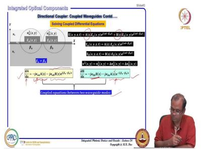
So, basically this A and B how they are coupled that actually will define the power or amplitude component or presence in waveguide A and waveguide B. So, this is something the first term and this is second term the first term you will note we have kappa aa and it is Az that means evolution of mode A in waveguide a amplitude A because of some kind of coupling coefficient kappa aa in that waveguide itself.
