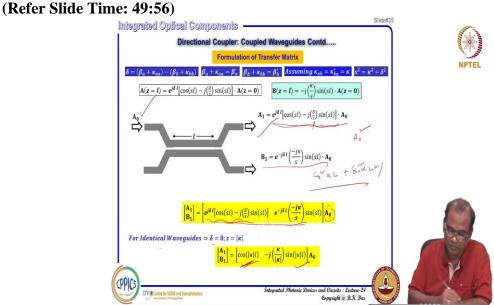
Now you see if I try to get a transfer matrix how it will be looking like I have only one input and I can have a row matrix so this is the value I have put first element and this is the second element. So, we can write A 1, B 1 something like this A 1 will be this one multiplied by A 0 and B 1 will be this one multiplied by A 0 that is in the matrix form we can write and if delta = 0 then it will be cos kappa l this one.
