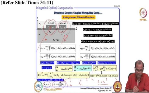
So, what we did let us consider an initial condition like this in waveguide a at z = 0 because you see this is z dependent waveguide z propagating waveguide this also z propagating when you are launching here something a 0 amplitude but here b 0 = 0 nothing I am just considering then I tried to find out at z = 0 I will be putting Az will be equal to A 0 and this will be z = 0 this will be z = 0 if I put then what I will be getting R 1 = A 0.
