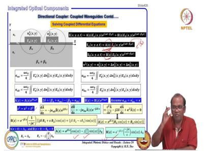
So, just introducing these 2 constant I get Az will be equal to this one the in this type of form and Bz it will be in this type of form I can write this is this is the ultimate solution. So, only thing is that in this waveguide what is unknown only unknown thing is that delta and kappa once you know delta and kappa is also known. So, kappa you can compute delta also you can compute so once you know numerical you can compute.
