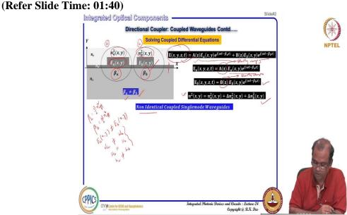
So, to solve coupled differential equation we just recap a bit how we got the couple differential equation we consider 2 waveguides they are parallel waveguides, waveguide a and waveguide b and this is a representative waveguide structure in silicon on insulator and n a square x y is the refractive index distribution to define waveguide a n square b x y that is corresponding to waveguide b.
