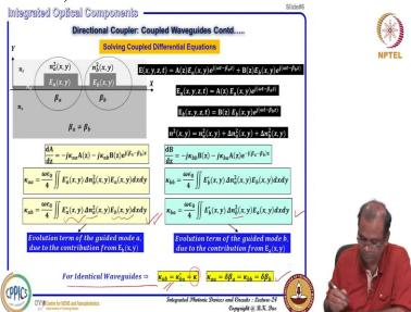
Now another coupling strength that is actually the term contribution coming from the second waveguide how much energy or amplitude even coupled contributing to waveguide a this is the kappa a, b that is actually defined if you see kappa a, b here E a star E b delta n a square we call this one something like that evolution term of the guided mode a due to the contribution from E b x, y.
