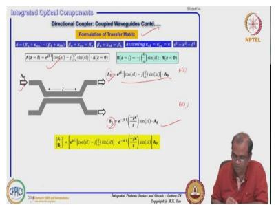
Now we are going for formulation of the transfer matrix I again repeat what is the amplitude whenever you are launching here you can get bar port amplitude and this is your cross port amplitude we represent A 0 and here we are writing A 1 and B 1. So, second waveguide any amplitude we are considering like a B and first waveguide any amplitude we are considering you remember that we are just considering Az and Bz.
