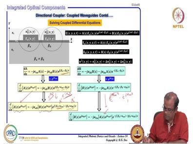
Now I just to do a little bit simplification so these one simplifying what I do left hand side I kept as it is right hand side what I did I just multiplied e to the power j kappa bb z and here I multiplied e to the power - j kappa bb z if you multiply these and these it will be basically one together. So, this one I multiplied with the b z I kept clubbed here just to make some kind of Az along with that e to the power j kappa aa here b z e to the power kappa bb I have kept.
