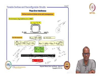
We have shown that ring resonator cavity this is the resonance condition we have discussed again and again. And this if you just this you concentrate here that beta = 2 pi / lambda m, m I have written that resonant wavelength mth order resonant wave length just to respect m here, n effective is the guided mode effective index 1 is the round trip length of the ring resonator and this is total length 1 perimeter length.
