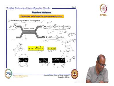
So, similarly if I just think about; another example of a directional coupler based powers splitters. So, as we saw before that a phase errors can actually deviate the output power in the
