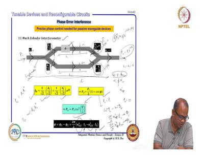
So, let us take an example of Mach Zehnder interferometer we have explained this before it is just a simple Mach Zehnder interferometer it is one input is here and you are accessing output here and this is you can be considered as a single mode waveguide. You know we know that any guided mode that can be defined as some kind of amplitude A and then E naught x y if it is a single moded waveguide field distribution.
