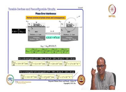
So, we have estimated simulated for a re-waveguide of W equal to this one 220 H equal to consider plus minus 10 nanometer variation can happen in slab thickness plus minus 20 this is just a old example, today you can get much lower values of course variations device layer thickness 220 nanometer plus minus 220 nanometer and whenever you are defining your waveguide in photolithography or even lithographic or advanced lithography system.
