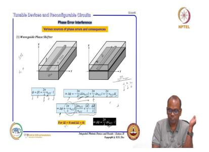
Let us see a waveguide let us consider a waveguide silicon on insulator waveguide and silicon on insulator waveguide you know one type of this is your box layer and then device layer is structure like a rectangular things in the top maybe top oxide layer is there and this is some kind of photonic waveguide structure it will have a diamond some like W and H but if you have a rib type waveguide structure like this then you can have a waveguide parameter will be W H and h.
