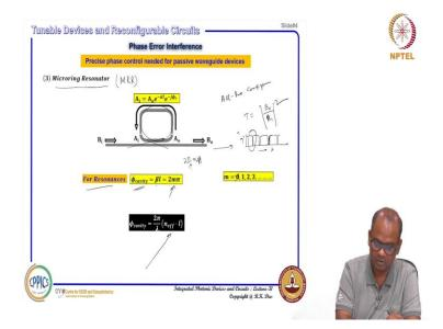
Now third important component and so I would say that the most important component for photonic integrated circuit called microring resonator sometimes we call it as MRR as you know in a micro ring resonator it is given the all pass configuration where you have a ring and one pass waveguide interacting where light will be tunneled here bit and round a pass again comes back in steady state you know that how to solve the transfer function.
