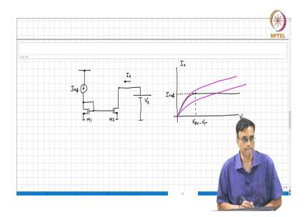
Now, the next thing we started looking at was various biasing techniques. Remember that the first robust biasing technique we looked at was the current mirror. So, this is some  $I_{ref}$ . So, ideally regardless of the voltage  $V_X$  as long as the transistor M2 is in saturation. What comment can you make about the current  $I_X$  is going to be?
