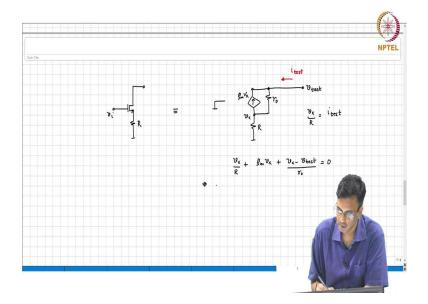
You set  $v_i$  to 0. So, this becomes  $g_m$  -  $v_x$  which is equivalent to saying this is  $g_m$   $V_x$ , this is  $v_{test}$ . The question is what is  $i_{test}$  ok? Before we do the math I should  $i_{test}$  be positive I mean should  $i_{test}$  be 0 or should it be still 0 I mean should it be 0 or non-zero?
