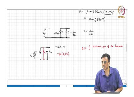
So, now the question is, well it seems like all along we have been working with an ideal transistor model which does not exist anyway. So, we now go back to all our circuits and start figuring out what this finite earlier transistor was an increment I mean was an ideal incremental voltage control current source meaning that the output impedance was infinite. Now, it is not infinite, after all there is some?
