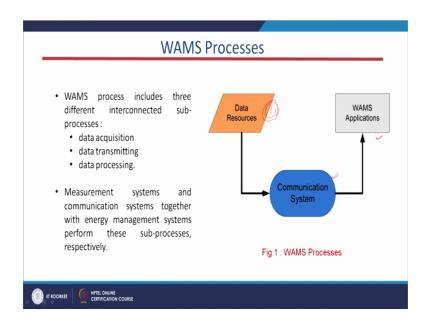
The first one is the data resources we will receive, this WAMS in WAMS technology the PMU basically send the data to the data concentrator PDC Phase Data Concentrator, there we will get the data resources and.
