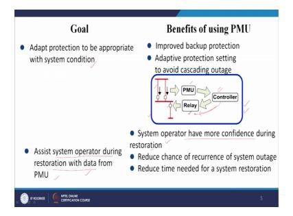
And the third one is adapt protection or adaptive protection to be appropriate with system condition, this adaptive protection means the protection is always essential for the power system where 5 percent of the total cost of the power system may dedicate for the protection of the system. Without protection, so we cannot save our equipments or lines or any a devises which are installed in the system.
