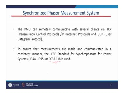
And the standard which is maintained for this PMU or synchrophasor measurement system that is basically the PC 37.118, this standard of IEEE is used to specify all the requirements or guidelines for the maintaining this PMU inside the wide area monitoring system. This is one of the synchronized phasorment system, the communication between this PDC and PMU.
