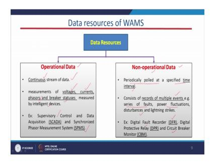
The first one is the operational data is continuous stream of data, it is a real time data it goes on it is basically measured at the end of PMU Phasor Measurement Units that is why it is very very vital component of the WAMS technology. Where we can measure the voltage current and frequency in the very bright flow like continuously we are just monitoring voltage current frequency of the system that is why it is a very continuous stream of data is possible there.
