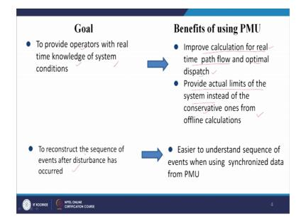
The first one is the, to provide operators with real time knowledge of the system. So, using this WAMS technology we are able to provide the real time knowledge to the operator who is sitting inside the control room that is important. Now using this information, real time information so what benefits we are going to get. The first one is improve calculation for real time path flow and optimal dispatch, if I know; what is the status of my power requirement.
