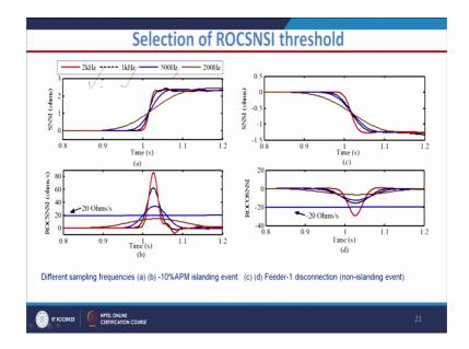
And how to select this threshold also we have studied very rigorously, where varying this sampling frequency 2 kilohertz, 1 kilohertz, 500 hertz, 200 hertz.
