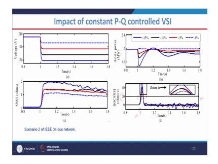
If you see here the rate of change of final figure, you could see here that this rate of change of super sequence current it exceeds the threshold, this threshold is 20 here and he exceeds the threshold value.
