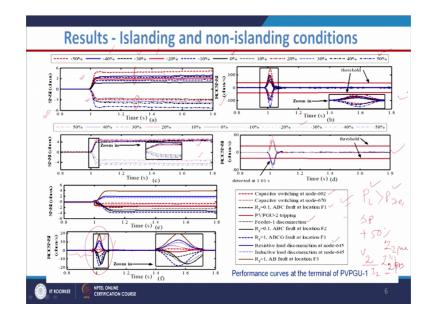
Here it is written S N ird is the superimposed negative sequence impedance right. So, SNSI SNSI stands for make Superimposed Negative Sequence Impedance. And he could see that for different positive result power mismatch like one is 50 percent, 40 percent, minus 30 percent and we went up to plus 50 percent. The variation is also I mean we did for 80 percent because of course, if we exceeds I mean if we be close to the higher percentage of power mismatch the factor is very good.
