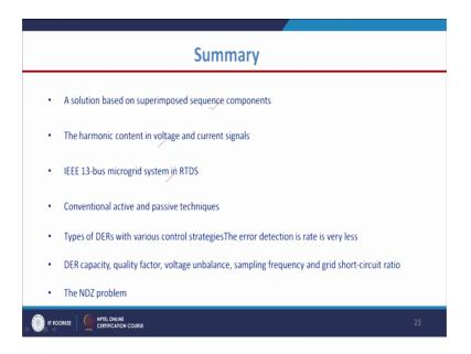
Now, in summary I will just discuss here that a solution we have provided here based on the superimposed negative sequence components and the harmonic, if present inside the voltage current signal by using a least error square base technique; we can always extract the fundamental voltage frequency phases. And in this case we have taken one 13 IEEE 13 bus system and also we have simulated 1 IEEE 34 bus system where we have also taken the tie line switches.
