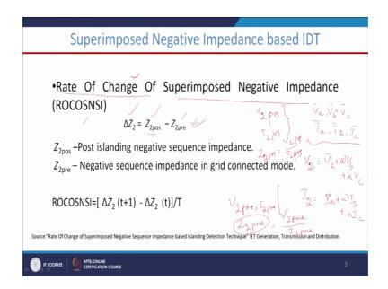
Here what we do the superimposed negative sequence impedance is going to be calculated first, the first step is we have to collect the voltage 3 phase voltages V a, V b and V c and also we have to collect 3 phase currents I, I b, I c at the terminal of the DGs or at the terminal of the DERs. Now, after getting this phases; you know we are calculating the phases as the terminal of the DERs using list error square base technique.
