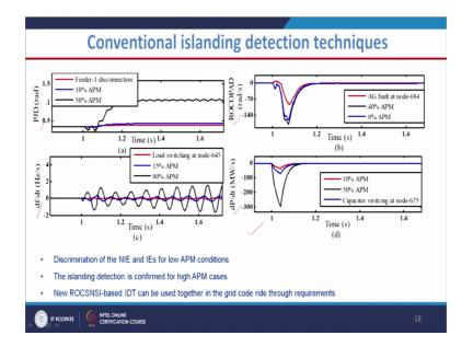
These are some of the comparison with the conventional techniques, this is for the rate of change of power and this is dP by dt and rate of change of frequency and phase jump techniques.
