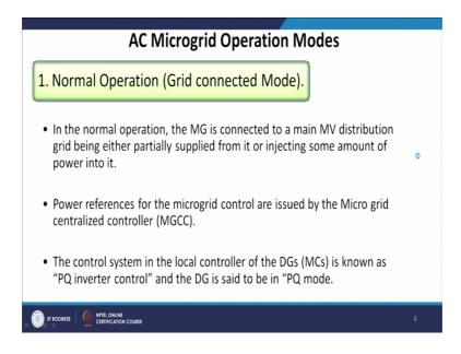
Now, in a normal operation the microgrid is connected to the main medium voltage distribution grid, being either partially supplied from it or injecting some amount of power to it. That means a microgrid which has been connected to your medium voltage distribution network, though it has its own generations to meet the local loads.
