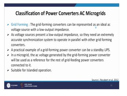
Now, classification of power converters AC microgrid; let us say grid forming the grid forming converters can be represented as an ideal AC voltage source with a low output impedance. As voltage sources present a low output impedance so, they need an extremely accurate synchronization system to operate in parallel with other grid forming converters.
