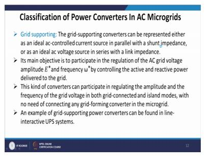
Now, let us move to the second one that is grid supporting. The grid supporting converter can be represented either as an ideal AC control current source, in parallel with the shunt impedance or as an ideal AC voltage source in series with a link impedance.
