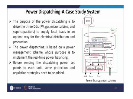
Now, if you look into the power dispatch scenario, the purpose of the power dispatching is to drive the three distributed generators to supply the local loads in an optimal way for the electrical distribution and production.
