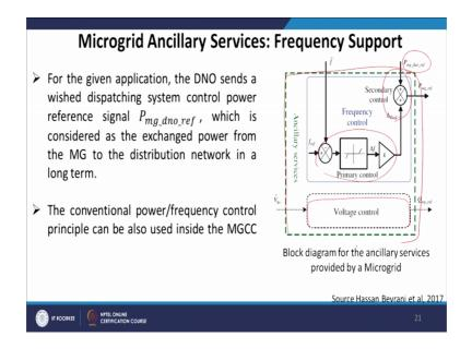
Microgrid ancillary services for a given application the DNO sends a wished dispatching system, control reference signal that is P mg dno reference which is considered as a exchange power from the microgrid to the distribution network in a long term. The conventional power frequency control principle can be also used inside the MGCC. Now
