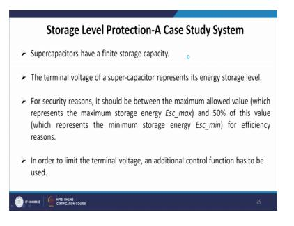
Now, storage level protection was quite interesting, where super capacitors have a finite storage capacity. The terminal voltage of a super capacitor represent its energy storage level. For security reason it should be between the maximum allowed value which represents the maximum storage energy and 50 percent of this value for efficiency reasons which represents the minimum storage. In order to limit the terminal voltage an additional control function has to be used.
