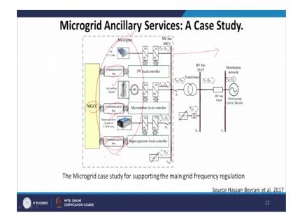
Now if you consider a microgrid ancillary services a very simple case study, especially to support the frequency regulation. Now you can see there is a distribution network and we have high voltage bus, and this is overly my microgrid where we have PV gas turbine, super capacitors they all connected to the grid along with MGCC through communication buses.
