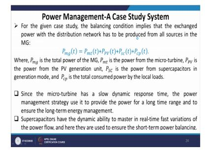
Now, if you wish to manage the power for a given case study the balancing condition implies that the exchange power with the distribution network has to be produced from all sources in a microgrid. Now the P mg the total power of the microgrid will be from the source as well as from the loads. So, it is power from the micro turbine, power from the PV generation, power from the super capacitor as well as the total consumed load or critical loads.
