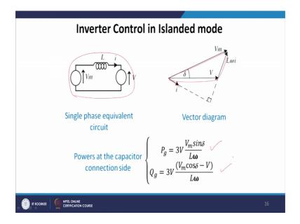
Now, in case of inverter control in islanded mode we can see the single phase equivalent circuit, and the vector diagram voltage lagging with its phase the drop and the final
