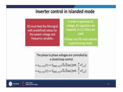
Now, the inverted inverter control in islanded mode distributed generator must feed the microgrid with predefined values, for the system voltage and frequency variables.
