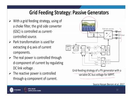
With a grid feeding strategy using of a choke filter the grid side converter that is GSC is control as controller source, park transformation is used for extracting DQ axis of current components. The real power is controlled through d components of current by regulating DC link voltage whereas; the reactive power is controlled through Q components of current.
