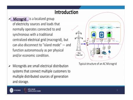
First of all we need to understand what is a microgrid. I mean microgrid do have different definitions, but one of the very basic fundamental way of explaining microgrid would be, microgrid is a localized group of electricity sources and loads that normally operate and connected to, and as well as synchronous with a traditional centralized electrical grid called microgrid. But can also disconnect if necessary to islanded mode and function autonomously as per physical and or economic conditions.
