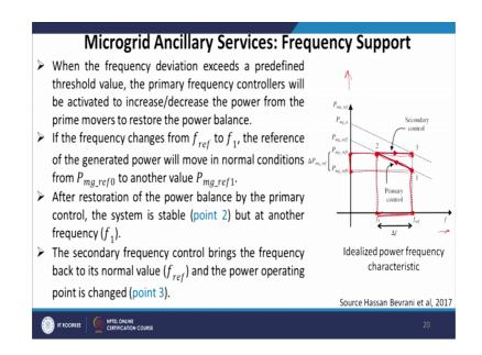
Now, if you look at when the frequency deviation exceeds a predefined threshold value, the primary frequency controller will be activated to increase or decrease the power from the prime movers to restore the power balance. If the frequency changes from let me consider this diagram, now let us say if the frequency is varying from f reference this point to another frequency that is f 1 and now because the power during f reference was my P mg at this point.
