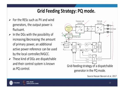
Grid feeding strategy for PQ mode of operation for the renewable energy sources such as PV and wind generators, the output power is flat fluctuant. In the DGs with the possibility of increasing or decreasing the amount of primary power and additional active power reference can be used by the local controller that is MGCC; now, the grid feeding strategy for a dispatchable generator in a PQ mode the block diagram, which has been shown in details.
