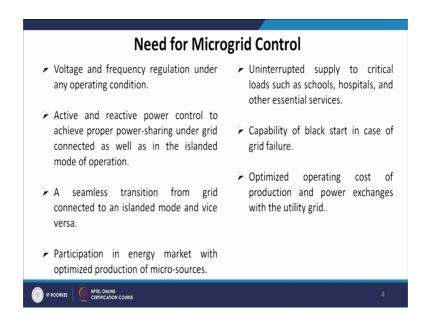
Now, voltage and frequency regulation under any operating condition is must, active and reactive power control to achieve proper power sharing under grid connected as well as in the islanded mode of operation is possible through microgrid controls. A seamless transition from grid connected to an isolated mode and vice versa.
