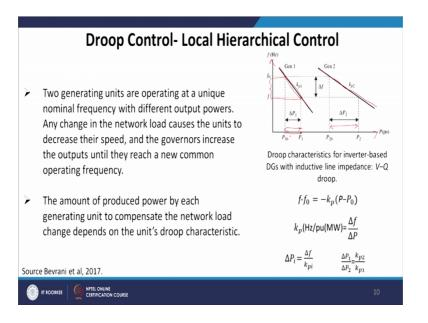
Two generating units are operating at a unique nominal frequency with different output powers. Any change in the network load causes the units to decrease this speed, and the governors increase the output until they reach a new common operating frequency. Yes we have to keep on changing until the both get the new common operating frequency, the amount of produced powered by each generating unit to compensate it the network load change depends on the units droop characteristic droop control.
