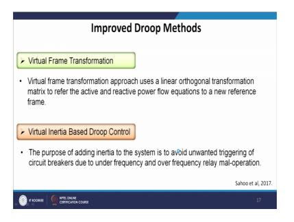
Now, in case of virtual frame transformation, virtual frame transformation approach uses a linear orthogonal transformation matrix to refer the active and reactive power flow equations to a new reference frame. Virtual inertia based droop control, the purpose of adding inertia to the system is to avoid unwanted triggering of circuit breakers due to under frequency and over frequency relay malfunctions.
