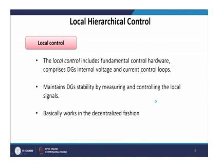
The local control includes fundamental control hardware, comprises distributed generation internal voltage and current control loops. It maintains distribution generators
