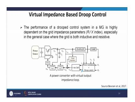
The performance of a drooped control system in a microgrid is highly dependent on the grid impedance parameters, that is R by X index especially in the general case where the grid is both inductive and resistive.
