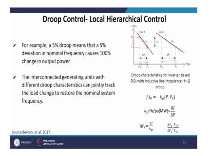
Now, let us try to understand the concept of droop control for example, the moment we say 5 percent droop means that a 5 percent deviation in normal frequency causes 100 percent change in my output power. The interconnected generating units with different droop characteristics can jointly track the load change to restore the nominal system frequency.
