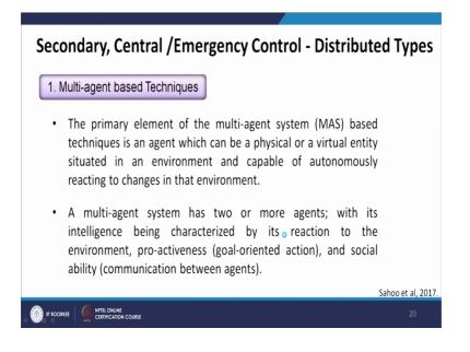
Secondary central emergency control distributed types, let us discuss on multi -agent based techniques, the primary element of the multi agent system based techniques is an agent which can be a physically or a virtual entity situated in an environment and capable of autonomously reaching to changes in that environment.
