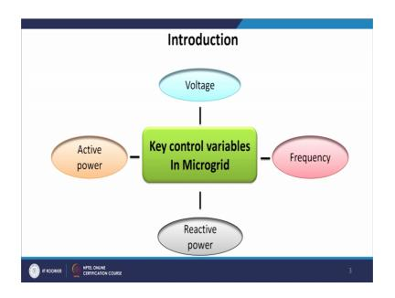
Now, the major key control variables in a microgrid is voltage, frequency, reactive power and real power. So, there is a whole 4 variables real power, reactive power, frequency and voltage decides the overall key control variables of a microgrid.
