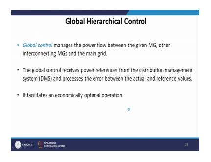
The global control manages the power flow between the given microgrid other interconnecting microgrids and the main grid. Now, the global hierarchical control is a step above where it manages the power flow between the given microgrid interconnecting to other microgrids. The global control receives power reference from
