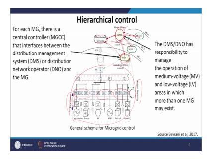
Now, getting deeper in to these, now this is my local control set up between my microgrid and do we have secondary control at each level. And now, the distribution network owner or operator that links to my microgrid 1, 2 and n and each microgrid will experience those secondary control as well as a local controllers and microgrid control connected to my distribution system and the signal may come from each and every individual microgrid controller from different microgrid through DNO.
