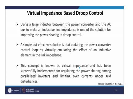
Using a large inductor between the power converter and the AC bus to make an inductive line impedance is one of the solution for improving the power sharing in droop control. A simple, but effective solution is that updating the power converter control loop by virtually emulating the effect of an inductive element in the link impedance.
