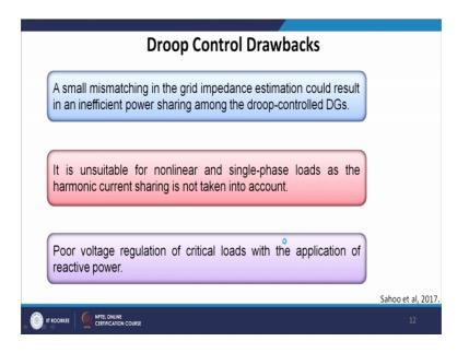
Droop control drawbacks, what are the major problems. So, the limitations of a droop control applications, a small mismatch in the grid impedance estimation could result in an inefficient power sharing among the droop controlled distributed generators. It is unsuitable for non-linear and single phase load as the harmonic currents sharing is not
