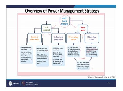
So, we can just have a quick look with the block diagram this is the key and it could be either grid connected or standalone and the grid connected either dispatched power or un-dispatched as we discussed and standalone could be DC bus voltage control or AC bus voltage control.
