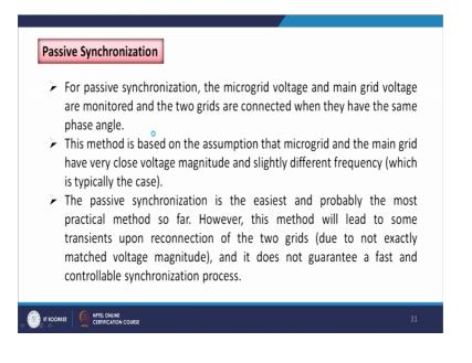
In case of passive synchronization the micro grid voltage and main grid voltage are monitored and the 2 grids are connected when they have the same phase angel. So, these 2 are monitored when they have the same phase then they are allowed to get connected in case of passive synchronization.
