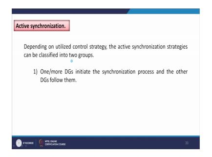
Depending on utilized control strategy the active synchronization strategy can be classified into 2 groups, first one or more distributed generators initiate the synchronization process and the other distributed generators has to follow. Second one all distributed generators take part in the synchronization process simultaneously.
