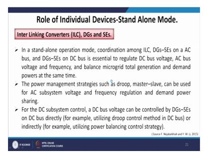
Now, during stand-alone mode of operation or islanded mode of operation how those devices interlinking converters distributed generators as well as my storage elements play an important role. Now, the in a standalone operation coordination among interlinking converters distributed generators and storage elements on an AC bus as well as the distributed generators and the storage elements in a DC bus is essential to regulate the DC bus voltage and AC bus voltage and frequency.
