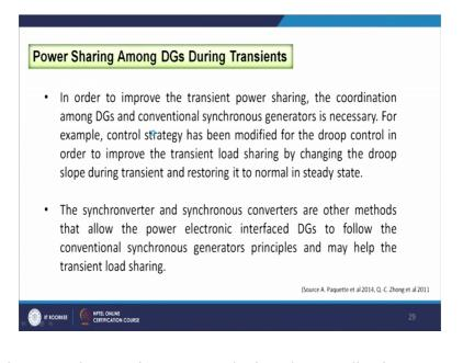
In order to improve the transient power sharing the coordination among distributed generators and conventional synchronous generator is necessary. For example control strategy has been modified to the droop control in order to improve the transient load sharing by changing the droops loop during transient and destroying it to a normal steady state value.
