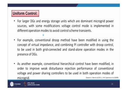
Now in case of uniform control for larger distributed generations and energy storage units, which are dominant micro grid power sources with some modification voltage control mode is implemented in different operation modes to avoid control scheme transients.
