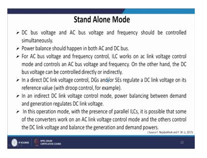
For AC bus voltage and frequency control interlinking convertor works on AC link voltage control and controls and AC volt AC bus voltage and frequency. On the other hand the DC bus voltage can be controlled directly or sometimes indirectly. In a direct DC link voltage control distributed generators and or the storage elements regulated DC link voltage on it is reference value for example, through droop control.
