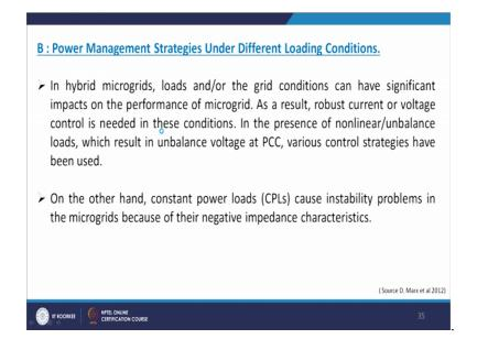
And in a hybrid micro grid loads and or the grid conditions can have significant impact on the performance of the micro grid. As a result robust current or voltage control is needed in this conditions, in the presence of non-linear unbalanced load which results in unbalanced voltage at my point of common coupling various control strategies have been used. On the other hand constant power load CPLs cause instability problem in the micro grid because of their negative impedance characteristics.
