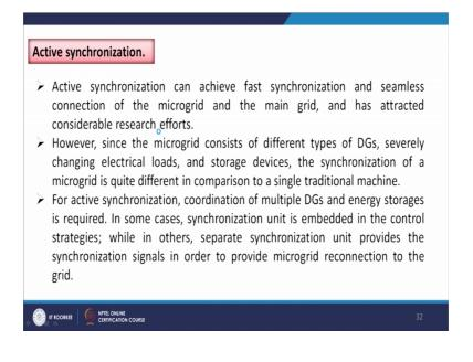
In case of active synchronization which is slightly advanced active synchronization can achieve fast synchronization and seamless connection of the micro grid and the main grid and has attracted considerable researcher effort today so any research related to active synchronization become a hot topic.
