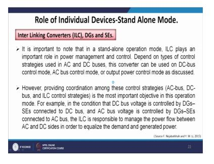
It is important to note that in a stand-alone mode of operation, inter linking convertors play an important role in power management as well as control depends on the type of control strategy used in AC and DC buses, this convertor can be used on DC bus control mode, AC bus control mode, as well as output power control mode.
