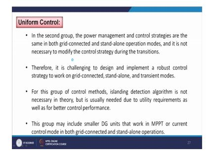
Now, in case of uniform control in the second group the power management and control strategies are the same in both grid connected as well as standalone operation mode and it is not necessary to modify any control strategy during the transition mode. It could be possible that you adopt to the same control strategy for both grid connected as well as isolated mode. So, that you need not change your control strategy trump a grid connected mode switching to isolated mode.
