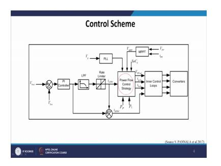
Now, the PFCS that is power flow control strategy we could see the power flow control strategy, where it extract the reference current based on operating modes and fed to inner current control loops. The pi controllers provide the duty ratio as output, which governs the input current a battery as well as ultracapacitor. Now, in case of GSC control loops the GSC control loop receives the reference from PFCS and operate accordingly based on it is mode.
