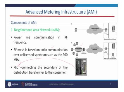
Now, I will come the function of this NAN. This NAN is basically it is a communication infrastructure and it may be a power line communication type or it may be radio communication type or it may also PLC the PLC stands for Programmable Logic Controller ok. So, it looks like this. The PLC looks like this programmable logic controllers are basically used mostly in industries to control the machineries. The operations of the machines and here also we can use the PLC concept by connecting the
