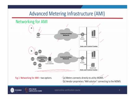
What is this figure a? The figure a tells that the meter, the smart meter is connected directly to the data control center or to the MDMS. So, which is this is the utility side and this is the customer side. This two meter basically this two devices like meters and the DMS are connected using a dedicated communication network. So, this kind of fashion of architecture or infrastructure is known as meters connect directly to the utility MDMS type. It is direct connection.
