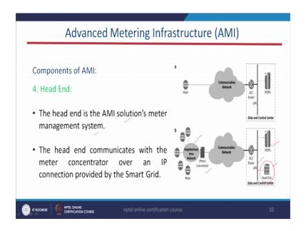
We already discussed, what is MDMS? What is this LAN and what is this meter concentrator and what is this NAN and the smart meters? So, another element or device, that is head end. This head end is AMI solutions meter management system. It manages the AMI solutions meter; whatever the data or information we exchange between the smart meter and this utility MDMS. So, those exchange I mean the data exchange should be managed properly. So, this data head basically does that ok
