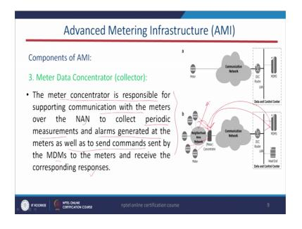
That is what I have just described in the previous slide and this is what written here. This meter concentrator is responsible for supporting the communication with the meters over the NAN to collect periodic measurements. This is important. It may be within 5 minutes 10 minutes. So, that periodic measurements and alarms generated at the meters as well as to send the commands or send the DMS to the meters and receive corresponding responses. I want to explain further, this point.
