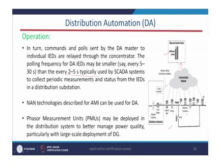
That is how the infrastructure already we have discussed. Here these are the devices like we have capacitors, we have recloser, we have distribution transformer, we have all these equipments and switches. So, this IEDs will send a data to this DA master control center. This is the DA master control center.
