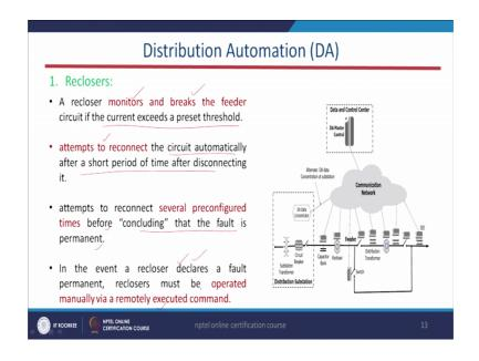
Now, basically the recloser is one of the component, one of the component components of the smart grid system and what is the function of it? Basically it monitors and breaks the feeder, if suddenly the current magnitude exceeds the set value or certain threshold value or it exceeds the predefined value.
