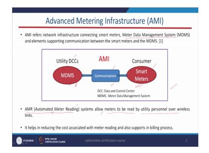
Coming to this AMI basic block diagram; you will see here that it consists of three components. The first one is the MDMS. This MDMS stands for Meter Data Management System and the second one is the smart meters which is basically a located in the consumers periphery or premises and this MDMS basically present inside the utility DCC's. And this is the data control centers which is basically present at the periphery or the premises of the utility
