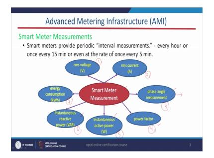
Now, the next will talk about what are the measurements we basically obtain from the smart meter. The first one is the RMS voltage and the second one is RMS current and third one is phase angle measurement. This phase angle basically we talk about the angle
