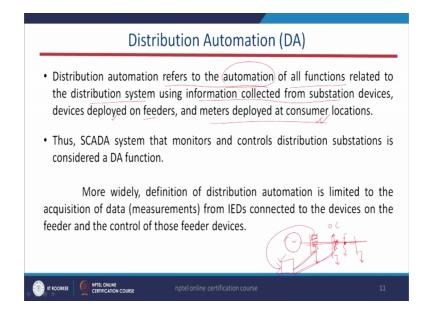
Now will come to the second technology and where also will talk about some components right so, the smart grid system that is our distribution automation system. So, as all of you know that the name itself suggest what? It is a basically automation system. The distribution system is basically automated as far as the operation is concerned; as far as the control is concerned, as far as the monitoring is concerned. It should be automatic in nature that is what this distribution automation.
