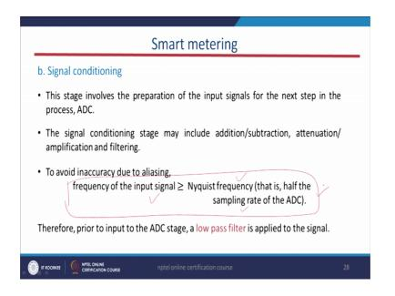
And signal conditioning as I said that this the Nyquist criteria we have here the frequency of the input signal. So, it will be greater than equal to the Nyquist frequency that is the half of the sampling rate of the ADC. These criteria we have to maintain while processing this signal from one block I mean to the ADC section.
