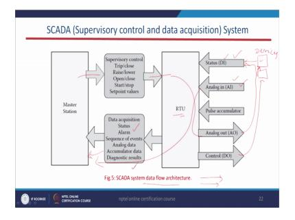
Now, this is the SCADA; system data flow architecture as I said that in case of a SCADA system we have RTU that is the real I mean Remote Terminal Unit or we call it also remote tele control unit, where it will just connect the data from the I mean from the different devices in the distribution system to the control center; main control center of the SCADA system.
