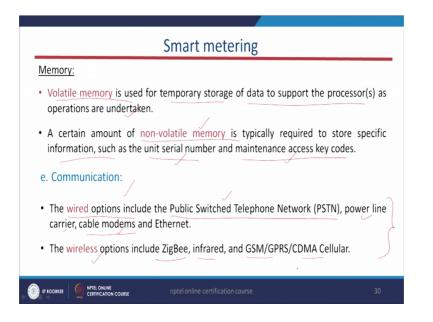
And this memory is used for temper use of the data to support the processor as operations are undertaken. And certain type of nonvolatile memory is also required to store specific informations such as unit serial number or maintenance access key codes; these two are important.
