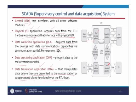
So, this remote terminal unit; what is the function of this? The main function of this is together the data from the field equipments and it will send to the master station. And before going in further the detail functions; what is this RTU? This RTU is basically, it is a microprocessor based device and that interfaces with the SCADA system by this transmitting the telemetric data to the master station.
