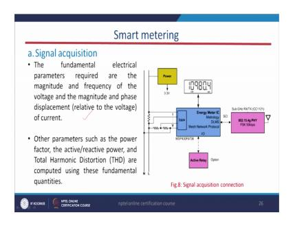
Now, this signal acquisition already we have discussed that the signal acquisition basically accuse collect the voltage current signals and then it further process to the ADC part.
