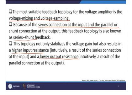
And that is the intuitive result of which we have already found out because it is a parallel, output is a parallel connections, output parallel connection primarily means that output impedance will fall down right and that is the reason you get a reduction in the output impedance.
