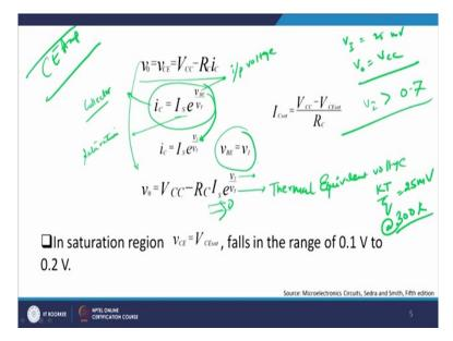
Let me give you the mathematical treatment here. So if you look very carefully  $V_0$  which is in front of you, right?  $V_0$  is there, right? If you look at  $V_0$ , this  $V_0$  is the output voltage and is equals to obviously  $V_{CE}$  must be equal to  $V_{CC}$  minus  $I_CR_C$ , remember? We have already discussed this point. My yesterday's talk or previous modules talks we have seen that  $I_C$  was
