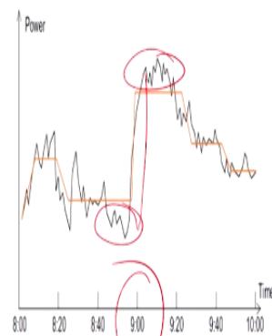
Fig.2 The principle of load leveling
