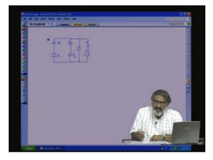
This is the diode, this is Th 1 and  $D_1$ ; then, Th 2 and  $D_2$ . Now, instead of having the freewheeling through the thyristor and diode, we will give a small low impedance path that will connect the freewheeling diode across here. Then we have the load; so here, how the conduction happens? Let us draw the waveform.
