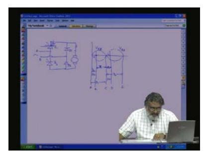
See, we will do it in a different way. Th 1, then for one limb, we will connect thyristor Th 1, Th 2. The other limb, we will connect the diode, here the load. So here, how is the conduction state? Let us draw the conduction with respect to our input mains AB. This  $V_{AB}$  and then this is the negative side that is  $V_{BA}$ ;  $V_{AB}$  and  $V_{BA}$ . Now, our firing angle starts from here, alpha. For the next device also firing angle starts from here for symmetry.
