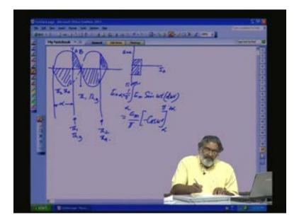
If you have axis here, this is our  $E_0$  alpha, the output voltage with respect to firing angle, this is our current  $I_0$ , then we can have operation in these two regions, two quadrant operation is possible. Now, let us find out what do the general output DC voltage equation where we are worried about the output DC voltage with respect to firing angle alpha. So, let us  $V_0$  alpha is equal to alpha to pi plus alpha Em sin omega t d omega t.
