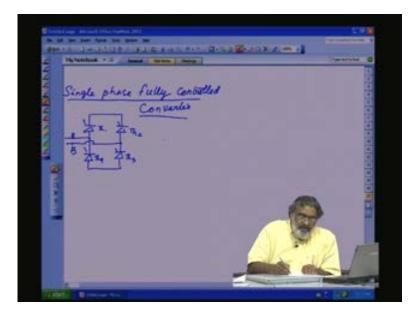
Now, thyristor 1 that I will mark it as Th 1, then you have Th 2, here you will have bottom also we will have controlled device that is Th 1, Th 2, Th 4 and Th 3. This is our mains, so here we will represent as a and b here, phase voltage  $V_4$ . Now, see here, all the 4 devices we can control. So, how we can get here positive as well as negative DC voltage? We will see now.
