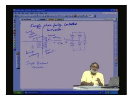
But many motor drive applications, we want 0 to positive as well as 0 to negative also that means the DC voltage should be variable from minus value to 0 to the positive value. Then what will happen to the quadrant region if you see in this figure with the voltage here?
