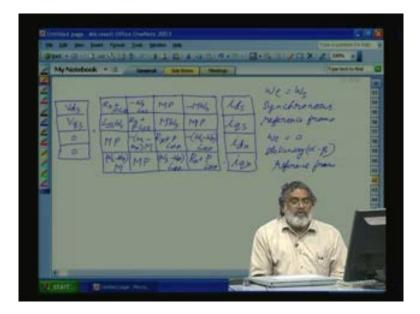
See we have, let us take omega rho is equal to omega s if you put it our dynamic equivalent circuit will be with respect to synchronous reference frame. Omega rho is equal to zero, then it will be stationary reference frame, stationary that means omega rho is equal to zero means dq will be aligned with alpha beta that is stationary alpha beta. the reference frame.
