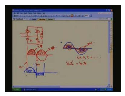
Thyristor, diode, thyristor sorry I will remove this one, diode, power load, again T 1, T 2,  $D_1$ ,  $D_2$ . Let us draw the input mains here. See, we are sequentially, we are coming to one point here. Previously, with the firing angle, the displacement keeps on increases with respect to the firing angle. Now, with semi convertor, we made that displacement, we have reduced to alpha by 2 that phi. Now, with the force commutation, we made that phi is equal to 0.
