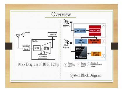
So, this is an RF energy harvesting chip based system; the there is one part which is the chip the other is indeed the complete system that they built. Inside the ship you will see that quarter wave match which we discussed is here, the impedance matching circuit is here and then what is inside the chip is an RF DC, usual Dickson charge pump that we
