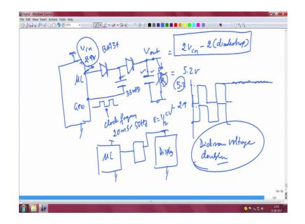
For this let me put back this picture to you I just quickly read drew that you have a microcontroller, and there is a GPIO pin on the microcontroller, and to this microcontroller what I will do is I will connect to one of the pins, I will connect the Schottky diodes these are basically Schottky diodes.
