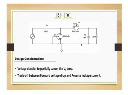
And essentially we are trying to exploit in silicon the fact that you can construct diodes from them these are all the w by l ratios, you do not have to worry so much about it. The fact that we are we have optimize the RF DC for a given frequency, this is very critical. When you say you are talking about RF DC, RF DC for what input frequency becomes important; so all these optimizations inside in silicon or for a given frequency.
