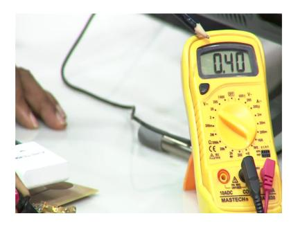
So, let me not load the capacitor and we will only make intermittent and measurement so that we can actually show you that it is building. So, what should happen? Soon as it builds to a little over 4 volts, you will see a data packet on this mobile phone. So, that is another important thing right now you can see that there is no data packet, there is nothing here it is blank and so, we need to ensure that now let us see how much is the voltage it is 3.74.
