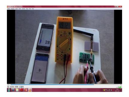
So, first let me. So, let me start this video. So, first is to. So, let me let me restart this video. So, here is a RFID reader that you see here which is throwing energy RF power on this antenna, this is a quarter wave match antenna impedance matching system, and the chip is right here you see the voltage being red there right you see nothing here now you will quickly see something yeah there you see you get some value, the value of the temperature also has changed.
