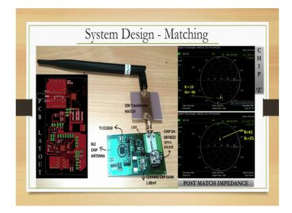
You can see this is the quarter wave match is a part and then this is the antenna receiving antenna the chip is here, embedded inside the microcontroller MCU unit is here, the BLE chip antenna is here, this is the PCB that we will we put together and you can see that quite nicely that is whole system seems to be working.
