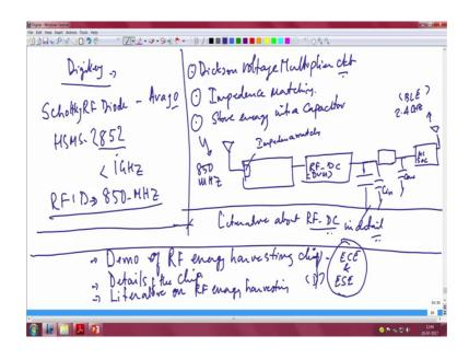
This from digikey easily, you can easily source this component from digikey, this is RF diodes it is an RF diode nothing, but a Schottky; it is a Schottky, Schottky RF diode these are also called detector diodes; this is from a company called Avago ok.
