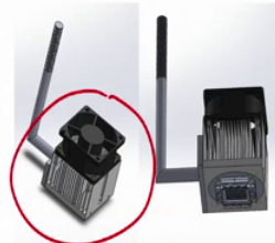
Figure: Design of UV exposure system with heat sink
