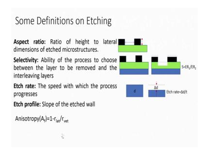
So, let us understand very important definitions on Etching. You can say parameters; you can say properties right; what are these properties? First property is Aspect ratio, what is Aspect ratio? Ratio of height to lateral dimensions of the etched microstructure. You can see here right, height to lateral dimension is an Aspect ratio; Ratio of high to lateral dimension of etched microstructures.
