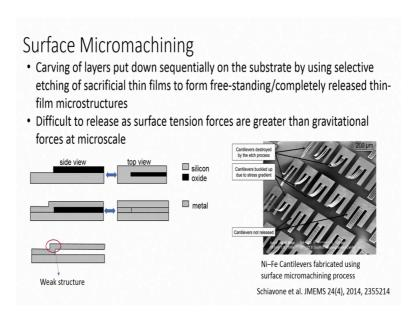
So, let us see what kind of structures, we can design or we can fabricate using Surface Micromachining? So, you can see here, this is an example of Surface Micromachining and if you see this example the gray colour is silicon and black colour is oxide. If you see the side view right, we have oxide on silicon.
