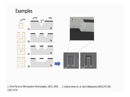
So, if you see the example here, you can see right V grew pyramid or truncated pyramid and these are cantilevers which are released, you can see here a completely released cantilever right and of course, this is taken from micro system technologies region by Prem Pal et al is just a schematic diagram. Also there is another paper that we have used from Johari J et al to get the idea of how the cantilever looks like, when it is released with the help of the etching technology right.
