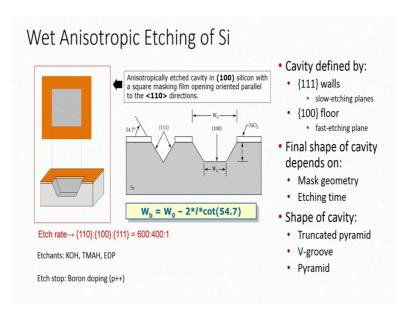
Now, when we are talking about isotropic and anisotropic etching, let us talk about Wet Anisotropic Etching, Wet Anisotropic Etching ok. So, you can see here that anisotropically etched cavity in 100 Silicon with a square mask film opening oriented parallel to the 100 direction right.
