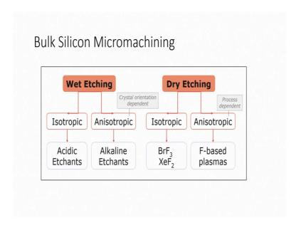
There is a Bulk Silicon Micromachining right; Bulk Silicon Micromachining. So, in Bulk Silicon Micromachining, we will see two kind of etching; one is a Wet Etching and another one is Dry Etching alright. One is Wet Etching another one is Dry Etching.
