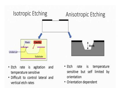
So, the one of the big problem in the isotropic in the etching world is the undercut problem right. So, you can see here isotropic etching and anisotropic etching. So, if we if this is the window, we want to etch this window. Then etch rate is agitation and temperature sensitive. So, here it will be temperature sensitive and depending on the chemical, difficult to control lateral and vertical etch rates right.
