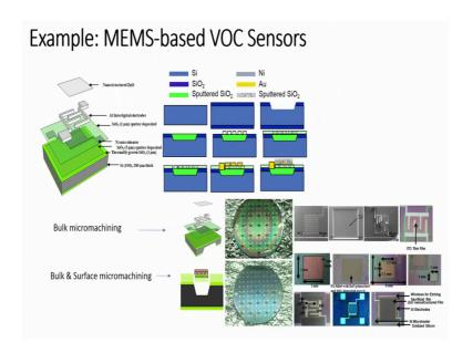
So, until now, what we have seen? We have seen that the micromachining can be 2 types; one is Bulk Micromachining; one is Surface Micromachining and then, we have seen how the Bulk Micromachining and Surface Micromachining can be used with the example of releasing a cantilever using Surface Micromachining.
