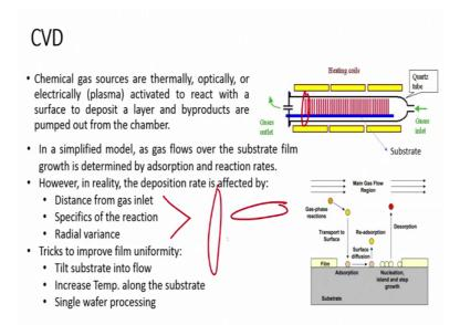
If you recall we have seen this kind of arrangement, sometime when we were discussing about wet etching wet oxidation and dry oxidation right, wet oxidation and dry oxidation. So, chemical gas sources are thermally, optically or electrically plasma activated to react with a surface to deposit a layer and by-products are pumped out from the chamber. So, we were introducing o 2 right it very high temperature about 1100 degree centigrade right. And the by-product was out of this particular Furness.
