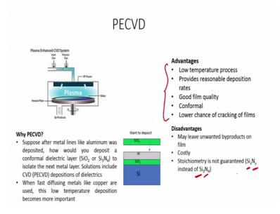
When we talk about PECVD so as we can see a system here is a heated plate there is a inert gas and process gas that we can inside in the system, is a R F power between there will be creation of plasma. And when the gas is reacts which is it will get deposited the film will get deposited on the wafer.
