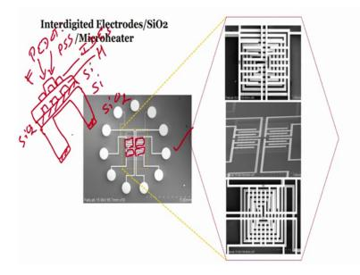
So, then what we have seen, we have seen an interdigited electrodes right. Then after interdigited, so in interdigited electrodes, what we have seen that there is a heater and on heater there is an insulator, on which there are I D E, patterns right. So, if you want to see interdigited electrodes, I will show it to you, I will show it to you here.
