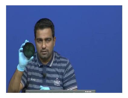
You can also hold the wafer in the way I am holding. It is similar to this right. Earlier wafer that we had was a micro heater right. So, there are two ways of holding it when you perform lithography, the best way of holding is always using tweezer.
