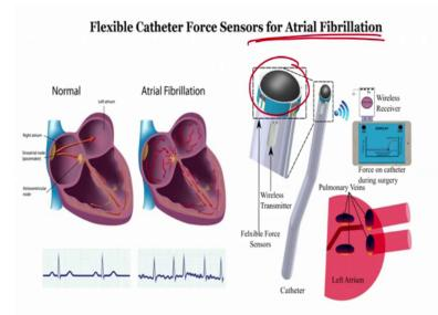
So, again we need a flexible force sensors right. So, I have to make a flexible force sensors and the tip of the catheter, at the tip of the catheter and I, I told you that we will discuss in detail Atrial Fibrillation. So, when we talk about tip of the catheter, then we need again a flexible force sensors right. So, what should be the sensing material? It can be just a strain gauge.
