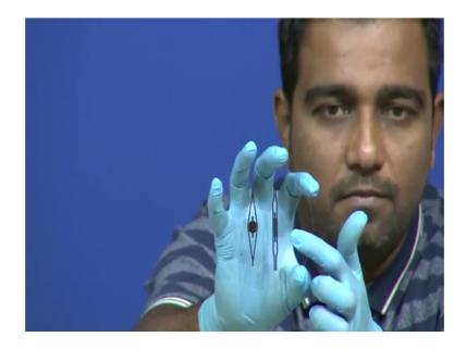
What I am showing it you is this one. So, this is the channel that we are looking on the S E M and then in between the channel, if you see the central region here, we can load the we can load the metrigel. On one side, we can load the cancer cells, on another side of the channel here, this device there are two channels, you can see right. So, one channel we can load the cancer cell another channel, we can load the epithelial cells or huec cells huec cells is a right way way, h u e c huec cells.
