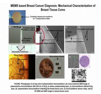
So, when we talk about piezoresistive cantilever right, I have told you that there is there is an s u 8 tip that is used for piezoresistive cantilever. And as a name suggests, there is a piezoresistor embedded within the cantilever piezoresistor embedded or integrated within the cantilever, right. How we can integrate a piezoresistor inside a silicon or a or on the cantilever we will see their factors.
