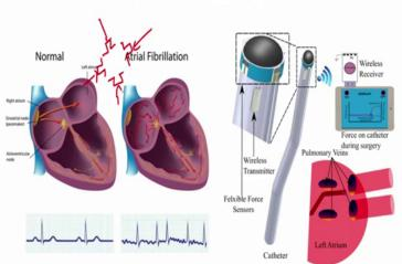
Flexible Catheter Force Sensors for Atrial Fibrillation
