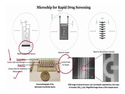
The electrodes for sure this these are used for impedance measurement which is given here the heater contact pads that we have just seen I have shown you the device and the contact pads are used to apply power so, that the heater can achieve 37 degree centigrade temperature right.
