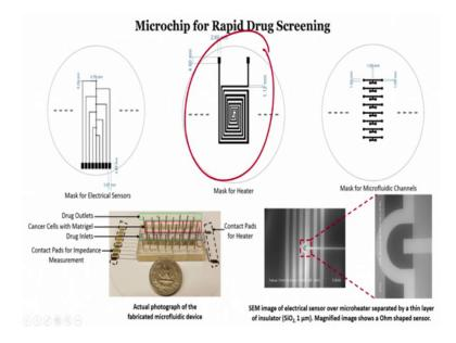
So, let us see one by one first step is we have to fabricate a micro heater right.
