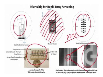
Over this micro heater, there is a insulator. On this insulator there are interdigitated electrodes. If I zoom in then I can see here each electrodes has a shape which is shown here right.
