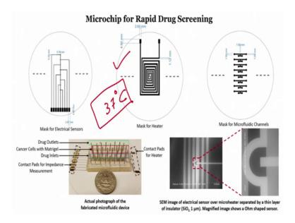
We have at the bottom at the first step is your micro heater or a heater why we require heater? So that we can achieve 37 degree centigrade for the cells to be alive right. So, we can keep cells alive, if we can have 37 degree centigrade temperature. Now, which is similar temperature to the incubator similar temperature the incubator?
