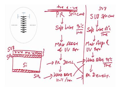
Next step would be soft bake, 91 minute, next step would be mask aligning mask align and UV exposure right next step would be PR developer, next step would be hard bake 120 degree centigrade again 1 minute on hot plate; this is our standard lithography process right.
