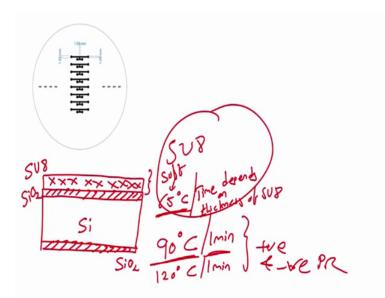
Now, for the prebake temperature is somewhere around 65 degree centigrade and depending on the thickness of SU 8 the time also varies right for positive photoresist and negative photoresist what we are discussing? We were discussing till now that the soft bake temperature or prebake temperature is 90 degree centigrade and if you use hot plate then you can heat it for or bake it for one minute.
