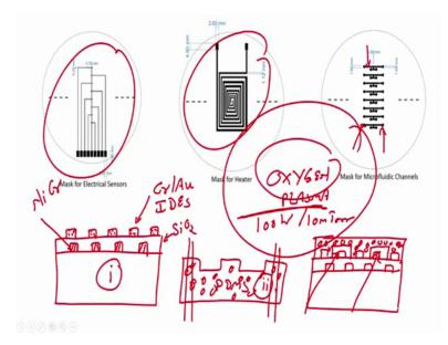
We have wafer one with interdigitated electrodes SiO 2 this is chrome gold interdigitated electrodes, which are this one right then we have silicon dioxide, then we have micro heater which is this one right and we have PDMS correct this is my second wafer 1 2 right. Now what I will do is I will perform oxygen plasma, oxygen plasma technique and after performing oxygen plasma technique I will stick PDMS to the glass.
