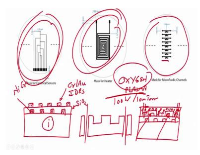
There is a hole there is a hole how can you create a hole? By using acu punch by using biopsy needle you can create a hole in the PDMS alright. If you have this then it is easy to connect the inlet and outlet or to lower the drug alright.
