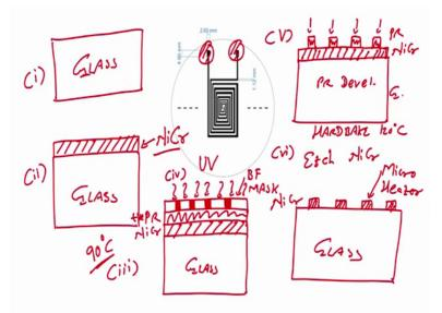
So, how can we fabricate a micro heater? N ow everything is on glass right. So, we take a glass, we take a glass and we deposit a metal for micro heater; let us say my metal is
