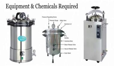
Autoclave: An autoclave is used to sterilize the equipment, utensils etc that are used for tissue culturing both for reuse and safe disposal. It is like a high-tech pressure cooker. It removes microorganisms like Virus, Bacteria, fungus, spores etc using high pressure and high temperature steam sterilization
