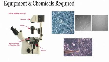
**Microscope:** Usually an *inverted microscope* is used inside a tissue culture room to look at the status of the cells that are being cultured. Different magnifications are possible like 10x, 20x, 40x, 50x, 100x etc. We use the microscope to see if cells have become confluent, how the health status of the cells is and when exactly to passage the cells. Inverted microscope gives better access for imaging of live cells.
