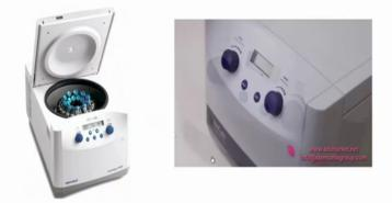
**Centrifuge:** This equipment is used to concentrate the cell suspension and remove the supernatant. The equipment has controls to set the required RPM and time of rotation. We can insert multiple falcon tubes at the same time. A sample video showing the operation is also given.
