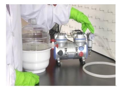
So, he has, we have a vacuum pump connected to the table. So, we will connect this tube through which air will be sucked out from the dessicator. So, as you can see behind the desiccator so, Suman will show you the vacuum pump. So, that is a vacuum pump, it is a portable vacuum pump which you can carry on around within the lab.
