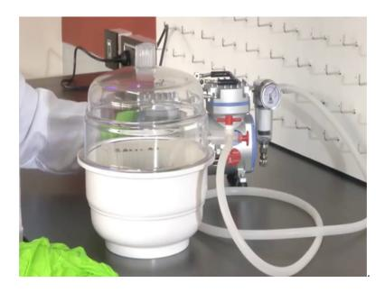
It has so, next to that pressure gauge the tube is connected, so, that tube will effectively go and connect to the desiccator. Now, Suman will connect that tube to the inlet port of the desiccators, you can see him connecting it. So, the red knob on top is the release valve. So, if he puts it in one position, it will allow the tube to suck out air. And once he puts in another position, it will lock the inside environment from the lockout inside environment from the outside world.
