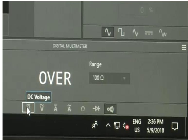
You can observe even measure DC voltage, it is similar to that of your normal multimeter, AC voltage, DC current, AC current, resistance measurement, diode checking, connectivity checking. So, everything can be done with single unit. Now, we will see how we are going to use this device and how do we measure using this particular software.
