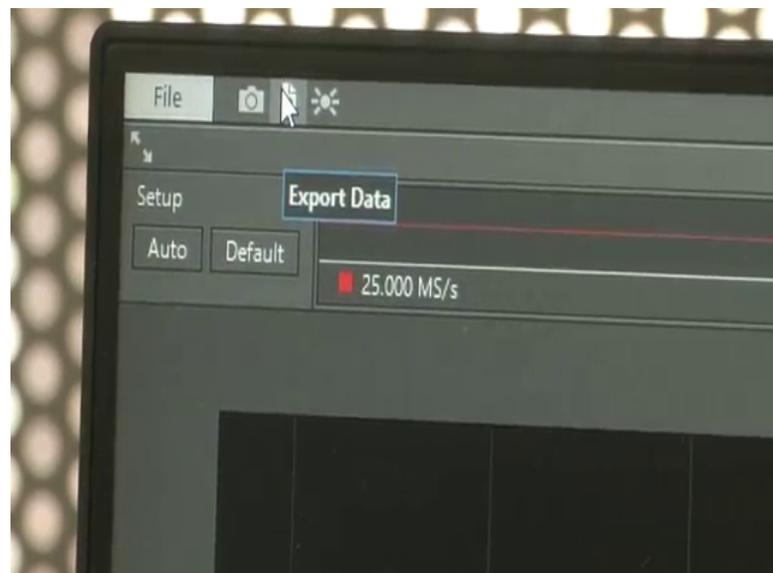
So, another advantage of this device is that whatever the data you are being acquired can be captured, the screen the screenshot of the system can be taken as well as the data, which is being acquired can be exported to a file also. Now, I will take what I do is that I will connect a multimeter units. So, this is a probe for the multimeter. So, I am connecting it to voltage low and another multimeter probe high. I just connected it.
