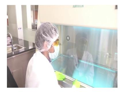
So, this bio safety cabinet provides that protection also. Ideally what we should do is that when assignment, we start using it we should switch off the UV light. So, there is we should switch off the UV light and use it, but then suppose we forget about it and we start using it. To start using it, we need to lift the lid. This is a glass lid that is provided for our applications.
