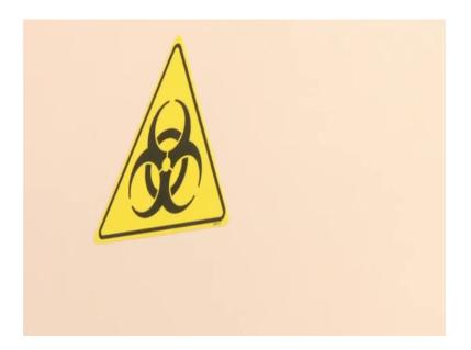
So, if you see the equipment, we have an emblem here yellow color. So, this is this is usually the sign for biohazard. So, what this emblem means is that this equipment, it does not mean that this equipment is a bio hazard, what it means is that this equipment deals with things is used to deal with stuff that may potentially be a bio hazard.
