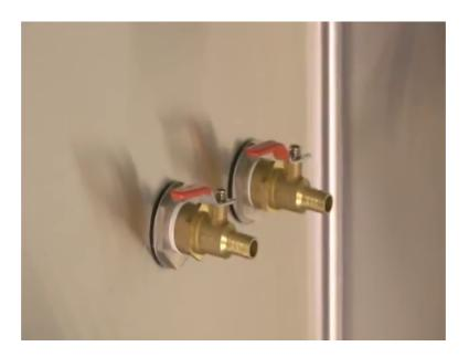
So, there are 2 nozzles. So, these nozzles can be used to supply deionized water or distilled water, very clear water and also to circulate air inside the bio safety cabinet.
