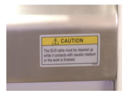
So, every time you finish the work, you should clean up this table with nice distilled water or even acetone or IPA you can wipe the surface clean it either when work is finished or while you are using any caustic medium and this is the safety limit that is provided. So, these are the major features that are available inside a bio safety cabinet. Shortly, I will show you after keeping some basic biology equipment inside how we have to actually work with things inside.
