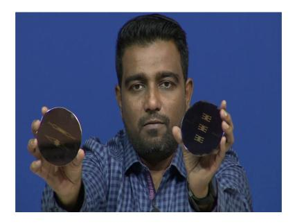
See this is how the silicon colour would be greyish. So, if I put now this one you can clearly see a difference when a oxide is grown right. Difference when the oxide is grown you can clearly see the difference in colour right, do not worry about the pattern just worry about the colour. Silicon oxide on silicon, very easily you can identify correct backside is oxide of course.
