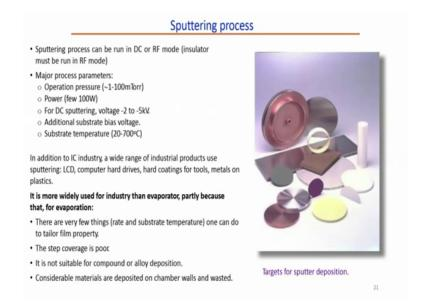
So, sputtering process like I discussed early can be run in DC or RF mode. Particularly when we are using insulator we have to use RF mode. The process parameters are listed here; operating pressure around 1 to 100 milli Torr power few of 100 watts; it is can be 200 watts, 300 watts. This is sputtering voltage minus 2 to minus 5 kilo volts.
