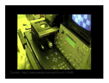
So, you ever do that to find the alignment mask, and then align them. So, once you have aligned them, we are ready for exposure. Then how do you expose, we press first your alignment check, which will bring it up to touch. You want make sure nothing moved, and then with some contact you hit exposure. And when you hit exposure, it is good to turn your back away from the light. So, does not damage your eye. So, hit exposure, and then we just turn away.
