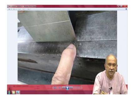
Now, having shared this machine, having done the marking; we now go onto the next operation saying, we have to get ready for bending. You see here, here if you see this is a folding machine and there is off course are long paper and then you can say this two lines are there and this is the clamping finger. What that clamping finger does is it holds the material underneath.
