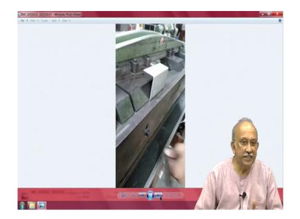
Can you see here, that make sure it is level; once it is level they after the bending limb is formed well, after it is formed is taking a try square and checking that we have a perfect 90 degrees. Can you see here, it has been bend twice; other direction also is checking this.
