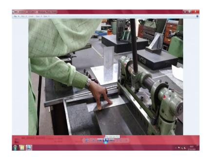
Advantage of this is; now this line is used for clamping it. Now, I will get back to this you see here we have, a developed length which has been calculated and is trying to share it to the necessary developed clamp. This is the open thing and mind you there are fingers here also which clamp it and much more important is, there is a straight edge and a back sharf.
