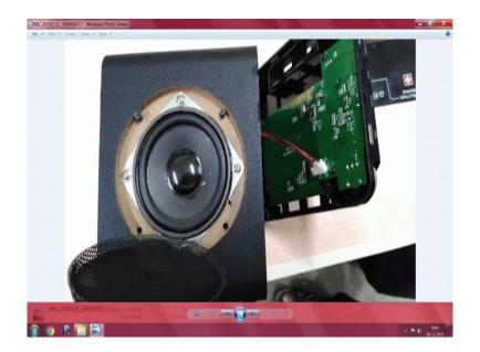
And on one of the faces when I open it, I noticed that they were just reduced it to half the thickness so, that a small speaker can be introduced.
