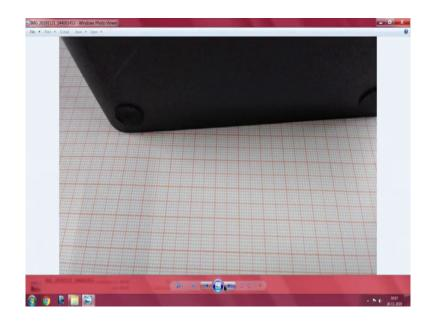
And this is where I wanted to tell you once more again and again, all you need to do is have a graph sheet underneath. This has taken with an old our printed circuit board system by which we used to have the 1.27 millimeter grid system. Even today, most what you call printed circuit board or anything they the pads are all placed on 0.1 inch grid it has gone all the way to 0.05 and 0.025 grid pitcher. So, you have this thing at the bottom, ok.
