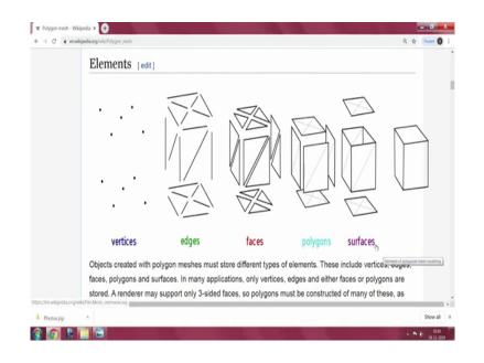
So, polygon meshes a same thing, a triangular mesh and ok. So, if you notice here the very basic things are this vertices, then we have the edges, we have the faces, then we have the various types of polygons and then we have the surfaces.
