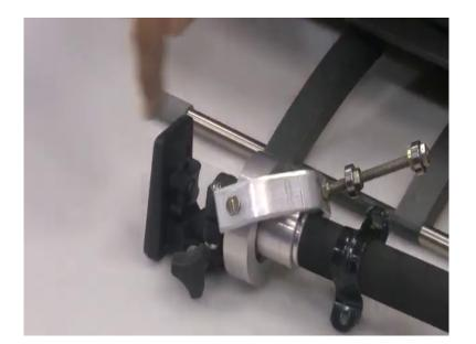
This is the vertical direction. So, I will call it the z axis. So, z axis this moves x axis, this moves and intentional layer removed the handle so that I can see the tiny small bearings. So, the outside diameter is 12 mm and the inside board is only 4 millimeters, I am sorry 5 millimeter. So, this whole thing now, the magic is everything here is off the shelf and everything here is completely interchangeable.
