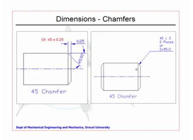
So, you see here coming back to the chamfers, it clearly says 45 degree chamfer; 45 into 3 at two places, 45 at this, this is a convention which is followed. Fortunately for us that is, those of us are moving out to the new CAD and we make a solid model; probably even if you were to miss the drawing can be read and the process people will be able to understand those things.
