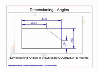
Next we come to how to mention angular dimensions. These angular dimensions are required depend on the particular type of job that we require. Sometimes for example, this looks like a chamfer in a corner or it could be a mating part. Say what they have written is, the remaining portion; after you remove that, the remaining portion is mentioned here, this is actually it is inches, but let me continue to just call it two and half millimeter.
