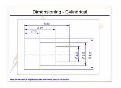
And when it comes to cylindrical dimensions you see a small difference is there; while this could be a sectioned view, half sectioned view and all this. Invariably these cylindrical parts are all mentioned with the diameter symbol, only in rare cases the word dia is written; otherwise depending on the precision you require two digits are all shown there. This looks like auto generated in some CAD packets; it is just mentioned it is AutoCAD in the beginning, probably it is done like this.
