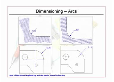
Now, here two other things here, there are two fillets here; this one is a fillet. Fillet is typically what you do for making sure that stress concentration does not occur. So, this could be part of a casting or it should be a part of some other thing, an internal bore. So, see where the thing is shown.
