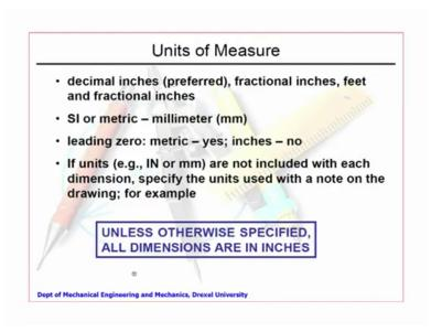
Next one talks about the basic units of measure; this is where the difference between any CAD drawing and physical prints make a lot of differences. One of the difficulty is until a print is made or job continues to be in some drawing units which in the end we need to convert it to a printable form. And in print form, the dimensions are picked from there and they are measured.
