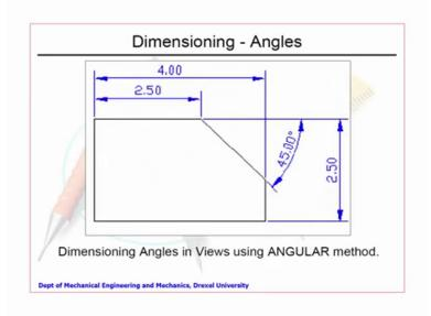
Then in some conditions angular dimension is preferred. And in some even other rare cases, if it is a taper, both the taper angle or the taper step is mentioned here saying; in this case both is one and half by one and half. Instead it will say 1 is to 1 with the other dimension saying, how many millimeters down it is for a given length, which is another way of representing those things.
