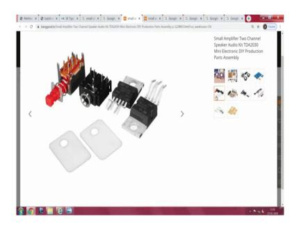
You have seen this these transistors and you see, how the leads have got offset and you see this small insulating thing. And, this thing gets fixed on these heat sinks. So, they are important, because in the basic simple circuit diagram very rarely, the heat part of it is shown here. And, all of these old things in end up with having a transformer for the power supply of lead things are becoming slightly different.
