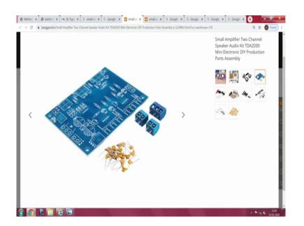
One of the first thing you will notice on the printed circuit board is there is a mask here, loosely it is called silkscreen mask and outlines of all the devices, which need to be fixed are all kept there. So, when you go here you will know where this goes this three pin device probably goes here ok. And, then these two what you call two pin terminals probably one goes here and one goes there.
