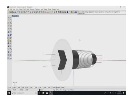
So, I have an advantage in case I want to make a hexagonal headed fastener, I can use this as a hexagonal head.
