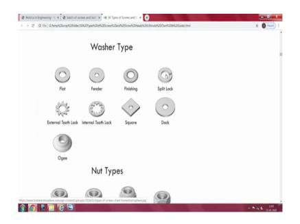
Now, we come to this large number of washers. A washer is used for several purposes, one of the simple flat washers like these are meant for just spreading the amount of force that it goes and then while you turn the head. The head should not score of the basic raw material. And, we have the other two things, we have internal lock what you call locks washer, external lock washer, then we have all sides of there is a split lock washer.
