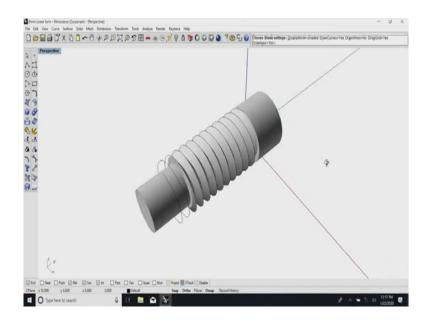
And, this cylinder here represents the root diameter; this cylinder here represents the outside diameter.
