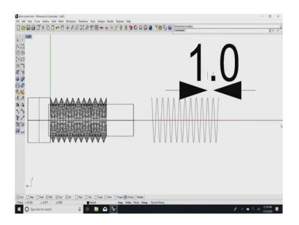
And, if you see the pitch it is 1 m m. These are the metric standard; metric standard almost refers to fine threads. And, generally in our electronics we use the threads from maybe around 0.5 or 0.6 mm all the way to around maximum 10 mm.
