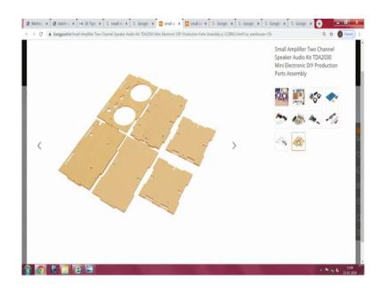
So, if I now go to this I am sure you know what it is it is nothing, but an acrylic sheet, that has been probably cut using a laser. The advantages of if you use a laser cutting device, you have to make a proper drawing once and you can always scale them open the way this parts interact.
